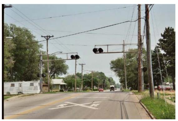
Standard Flashing Light Signals (No Gates) -- Ridgley Avenue in Springfield
